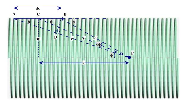
However compared to the magnetic field exerted by the whole solenoid, this magnetic field is very small. So it is denoted by  $dB_{ndx}$
