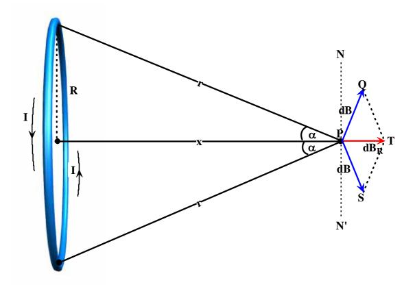
Similarly the magnetic field at 'P' due to 'dl' at the bottom is also given by  $dB = \frac{kIdl}{r^2}$  along PS.
