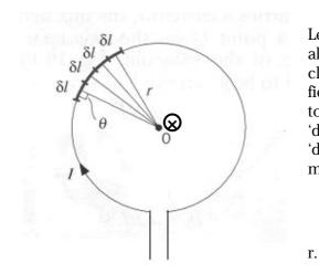
Let a coil be considered which is bent in the form of almost complete circle. Let a current I be supplied in clockwise direction which will give the overall magnetic field away from the observer at the centre 'O' (according to Fleming's Right-Hand Thumb rule). Let a small portion 'dl' be considered somewhere and a radius be drawn from 'dl' to 'O'. Then according to Biot Savart Law, a small magnetic field 'dB' given by 'dl' can be expressed as:
