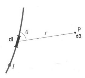
Since the portion considered is very small, the magnetic field given by it at point P will also be small. By experimental observations and empirically also, dB is found to depend on several factors.
