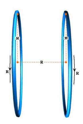
This means in the regions where the distance of a point from the coil is around  $\pm \frac{R}{2}$ , i.e. it is at a distance of  $\frac{R}{2}$  at both the sides, the magnetic field would be decreasing at a constant rate, i.e. it will decrease by the same amount for the same distance from the coil if taken away from the coil and increase by the same amount for the same distance from the coil if brought near.
