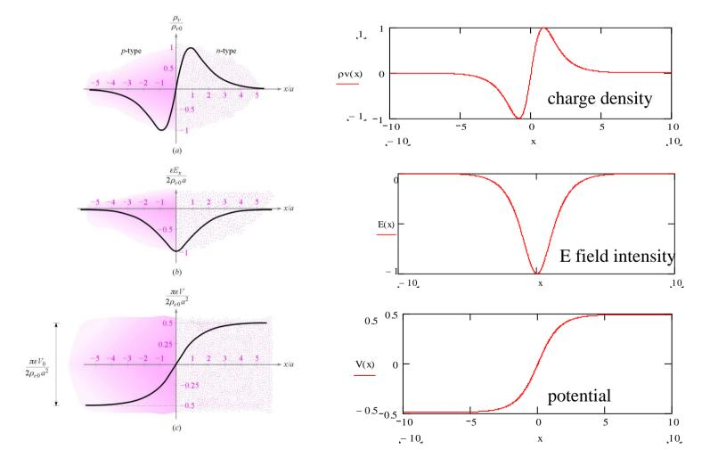
Referring to the figure below and the specific boundary conditions for the potential on the sides of the structure ...
