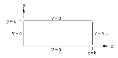
... choose the dimensions a and b of the box and the otential boundary condition<sub>0</sub>V
